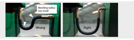
If the installation conditions allow, the bending of a hose line should start after a straight section with a length of 1.5 times the outside diameter. If necessary, kink protection or similar must be provided in such cases.
