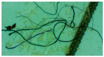
100x magnification of a sample of unfiltered HLP 46 fresh oil as supplied in a canister
