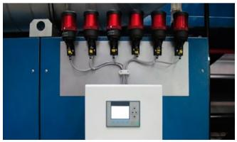
Control of water sensors on a plastic injection moulding machine
